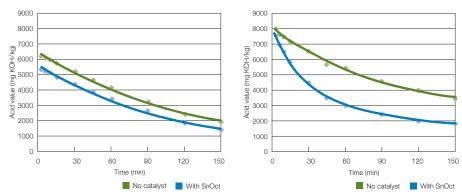
Different acids show diverse reaction kinetics with Cardura<sup>™</sup> E10P acid scavenger. Catalysts can have a positive effect on the reaction rate. Cardura<sup>™</sup> E10P acid scavenger enables base stock producers to reach very low acid value levels in a short period of time, which saves production time and energy. Furthermore, ester oils with a lower acid number are less prone to hydrolysis.
