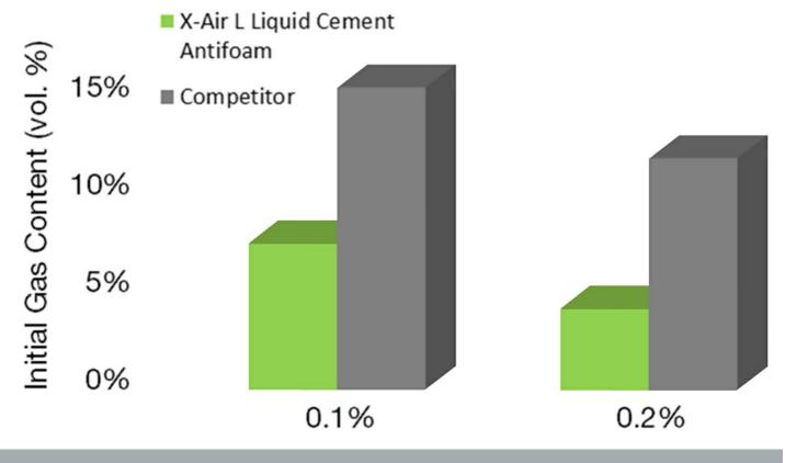
The X-Air L liquid Cement antifoam is over twice as effective as the competitor at 0.1% and almost four times as effective at 0.2%
