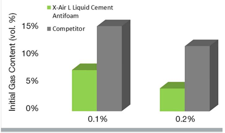
The X-Air L liquid Cement antifoam is over twice as effective as the competitor at 0.1% and almost four times as effective at 0.2%
